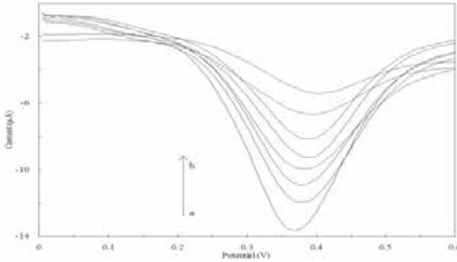
DPV curves were separately scanned to record the current response (Fig 4). When *M bovis* was captured by the anti-*M.TB*/ALP-IgG/AuNPs/*Ch* biofilm on the electrode, there would be an additional layer, which became a barrier for partly shielding the active center of immobilized ALP-IgG and decreased the catalytic capability of ALP.22 Consequently, a significant decrease in the DPV peak current was observed with the increment of *M bovis* concentration (Fig.3).
