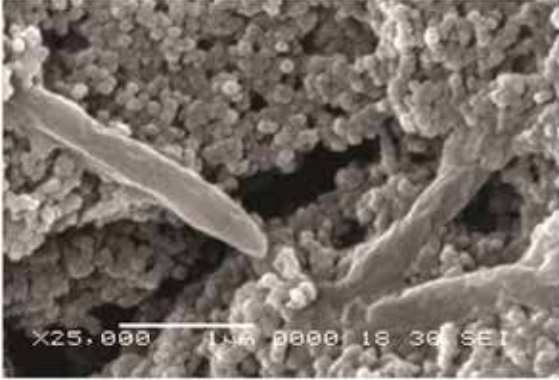
Figure 2. Scanning electron microscopic image of magnetic nanoparticles to capture M. paratuberculosis .
