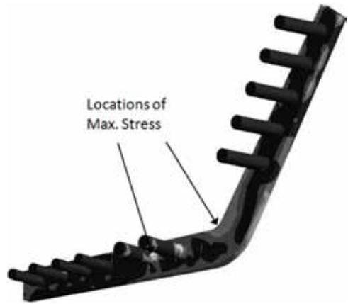
Figure 5: Stress Concentrations In the Implant In the Lateral Configuration Indicating Localised Failure of the Implant Material which would cause failure of the plate and screw heads to shear off
